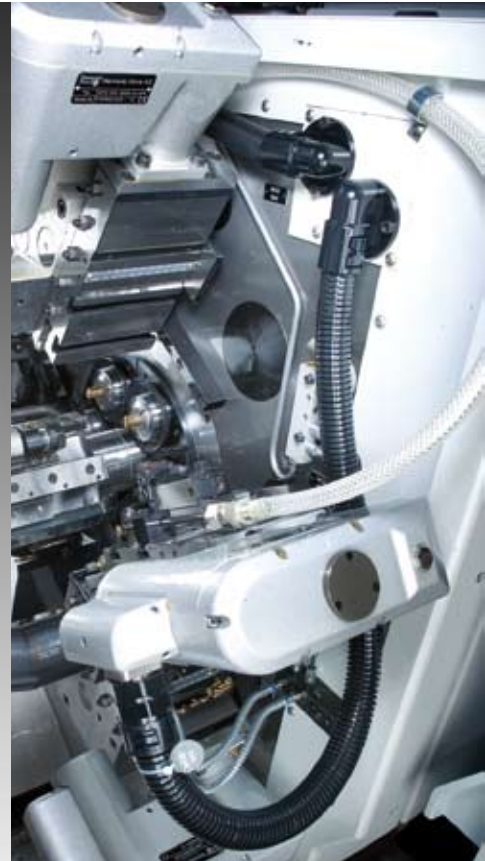
Motorised cross slide fine adjustment for the correction of dimensional errors and for tool wear offsets
