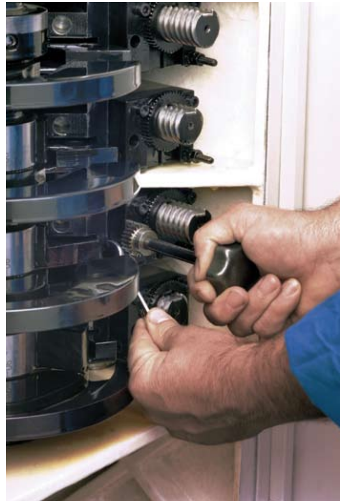
Setting an endworking slide rocker – infinitely adjustable and easily accessible
