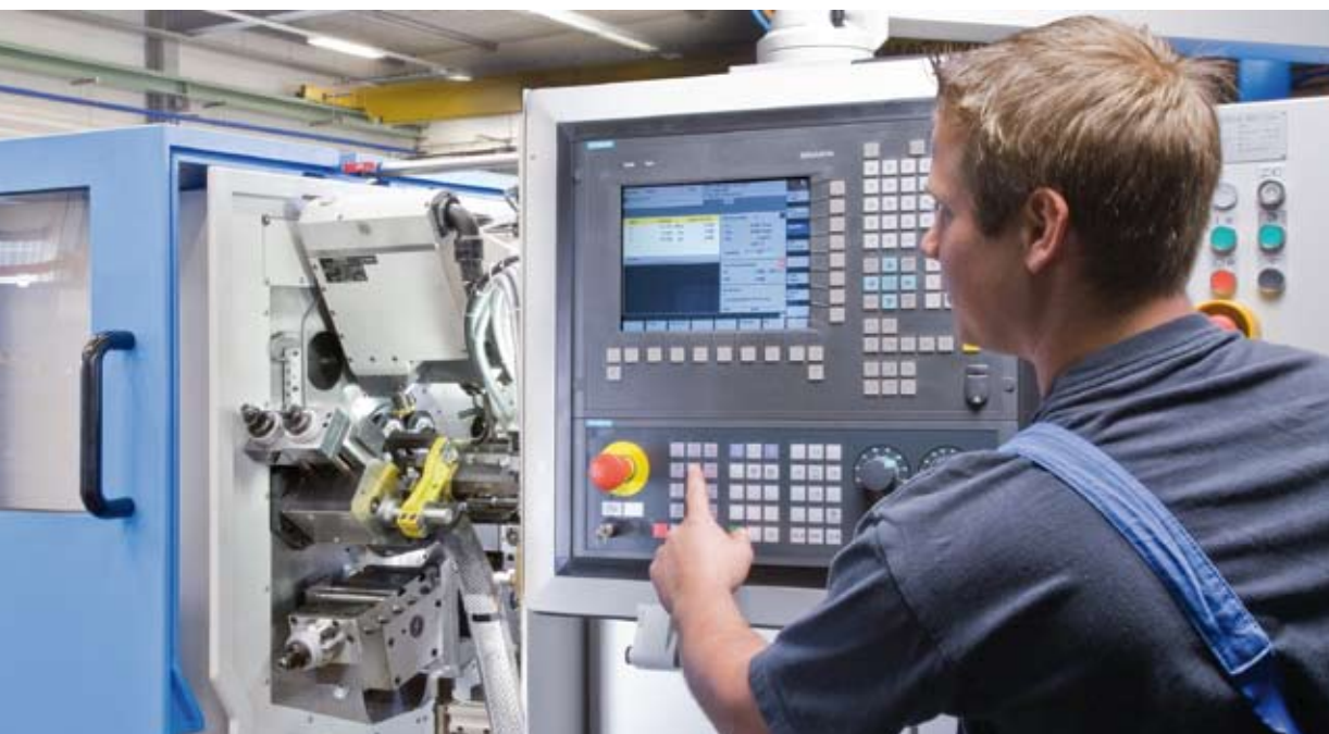
SG 18 and AG 20 – Cam-controlled multi-spindle automatics with options for CNC machining
