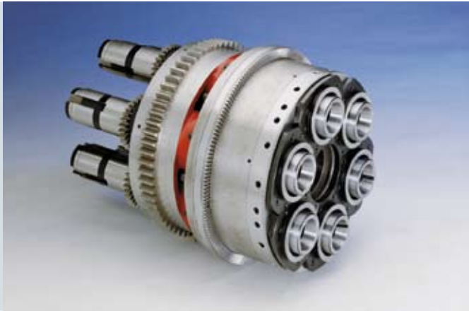
Spindle drum of a six-pindle automatic SG 18
