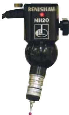
This is a sensor that collects the coordinate values of the surface of a workpiece which the stylus contacts. Various interchangeable styli are available to suit the task in hand: such as ball styli with various diameters, and others with specially shaped tips to best meet the requirements of a large variety of workpiece shapes and evaluation methods.
