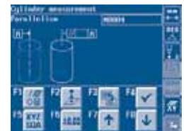
**Step 4:** Press the **F4** key to show the calculated angle between the axes.
